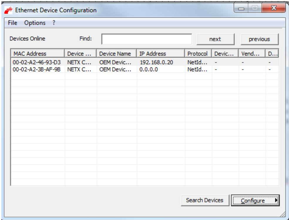
Since 192.168.0.20 is the factory IP address for the laser, connecting additional lasers and searching at the same time will result in IP addresses of 0.0.0.0 for the additional lasers. Their IP addresses can still be set without any problems.
