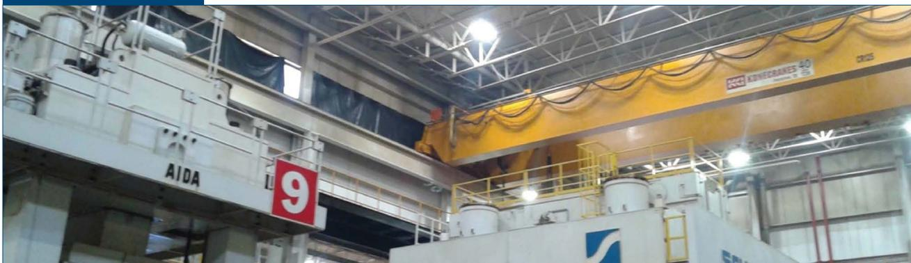
*Overhead crane over a stamping press, which usually is made into a no-fly zone.*
