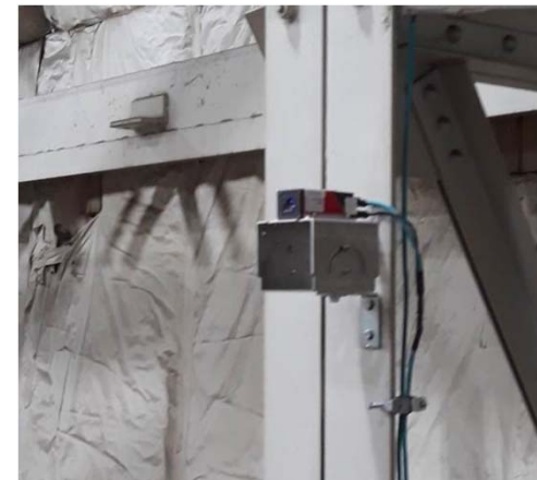
Laser sensors mounted on building column
